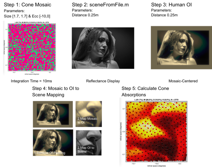
Figure 2: Pipeline for generating scene-absorption training and testing sets using ISETBio tools
