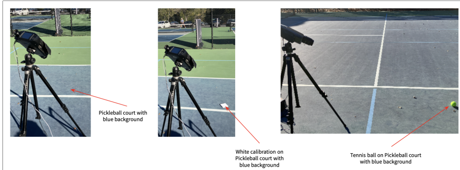
Figure 7: Pickleball court with a blue background, white calibrator, and tennis ball in sunlight
