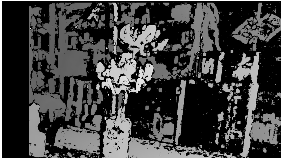
Figure 13. Optimal result (with numDisparities=176 and blockSize=21) of StereoBM, with 12.0 ms latency, 1.68% error rate and 34.56% recall.
